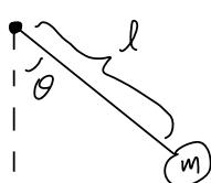
By conservation of energy, the motion of pendulum is periodic, and when  $0 < \theta_0 < \pi$ ,  $\dot{\theta}_0 = 0$
